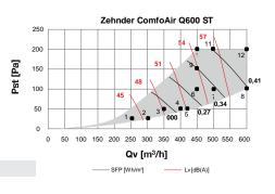
L<sub>w</sub> in dB(A) reference 10<sup>-12</sup>W, SFP [w/(m³/h)] calculated using data measured in accordance with EN 13141-7: 2010, ¹L<sub>w</sub> in dB(A); sound, supply air/extract air measured in accordance with ISO 3741 including end reflection in accordance with EN 13053:2006, ²Zehnder ComfoAir Q with G4/G4 filter and pre-heater
